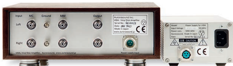
ABOVE: The low noise enjoyed by the VIDA phono stage is achieved, in part, by use of an outboard PSU. Separate MM and MC input RCAs are selected on the front panel. The single-ended outputs, also on RCAs, are fixed rather than volume-driven
